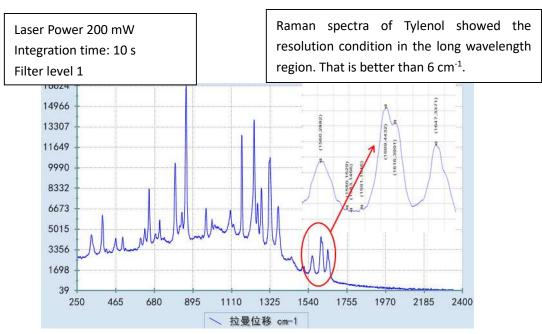
Fig. 2.2 Raman spectrum of Tylenol, the vibration mode 1610/1615 cm<sup>-1</sup> can be resolved.
