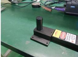
Fig 2 Fluid sample cell (Liquid chromatography bottle) (Optional)
