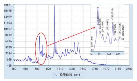
Fig. 2.3 Raman spectrum of petrol 93#, the vibration mode 723/732/742cm<sup>-1</sup> can be resolved.
