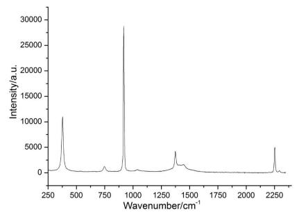
Figure 1 Raman spectra of acetonitrile
